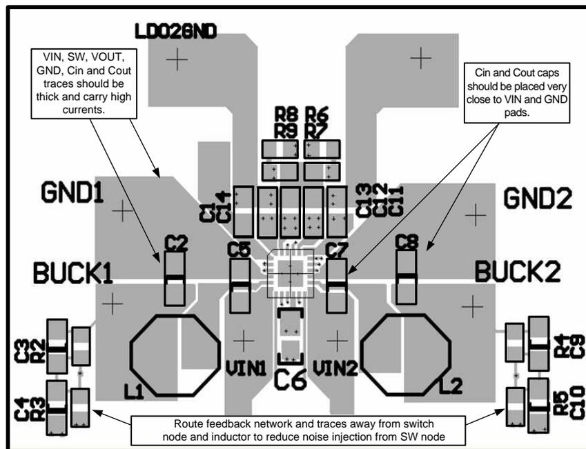
Figure 32. Board Layout Design Rules for the LM26480
