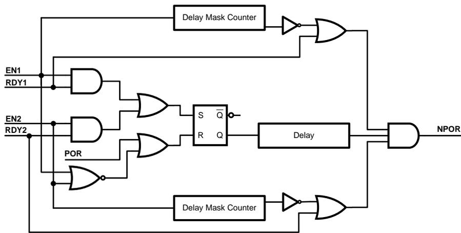
Figure 31. Design Implementation of the Flexible Power-On Reset
