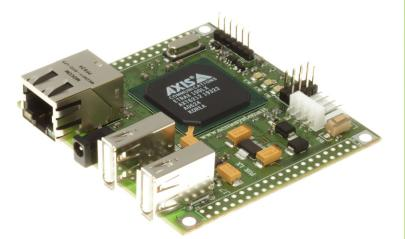
The FOX Board is an Embedded Linux Core Engine with reduced size and low power requirements especially designed to enables an easy integrate your design with standard LAN and Internet WEB protocols and applications.
